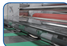
AUTOMATIC FEEDING GAP CONTROL DEVICE
