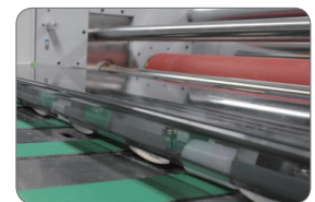
Automatic feeding gap control device
